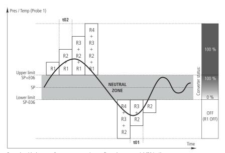
Example with the type of compressor rotation configured as sequential (E04=1)
